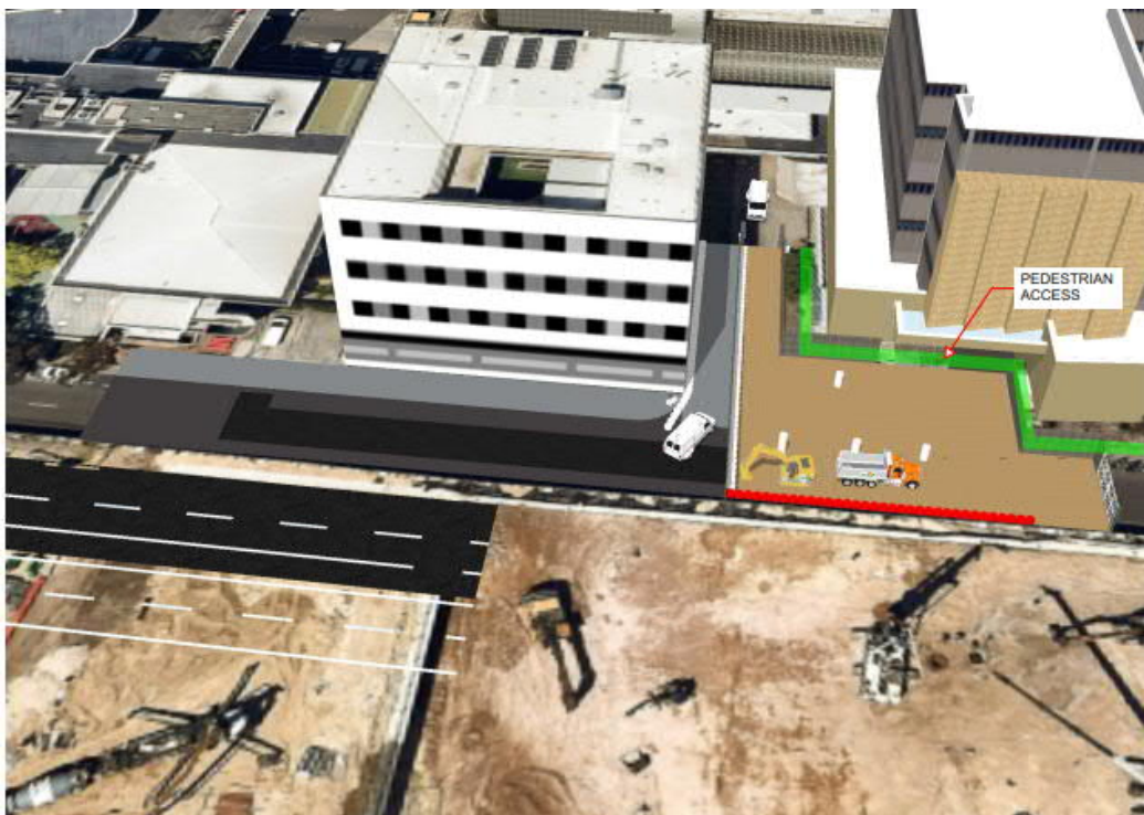
Figure 10 – South stage – Bulk excavation– stage 4 of 6
