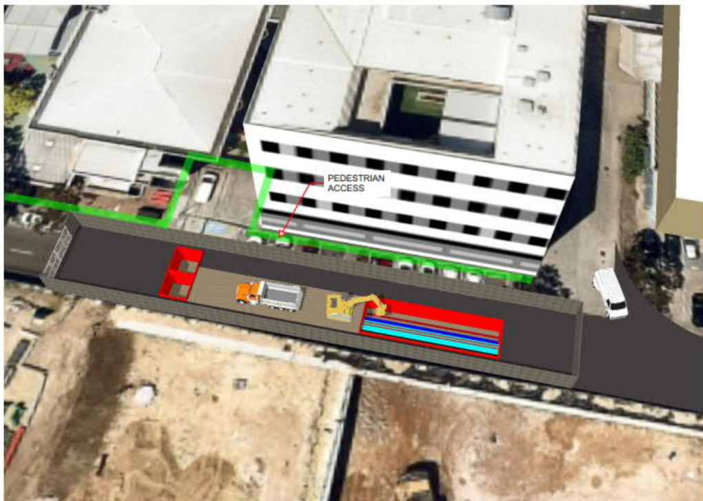
Figure 8 – North stage – services diversion – stage 3 of 6
