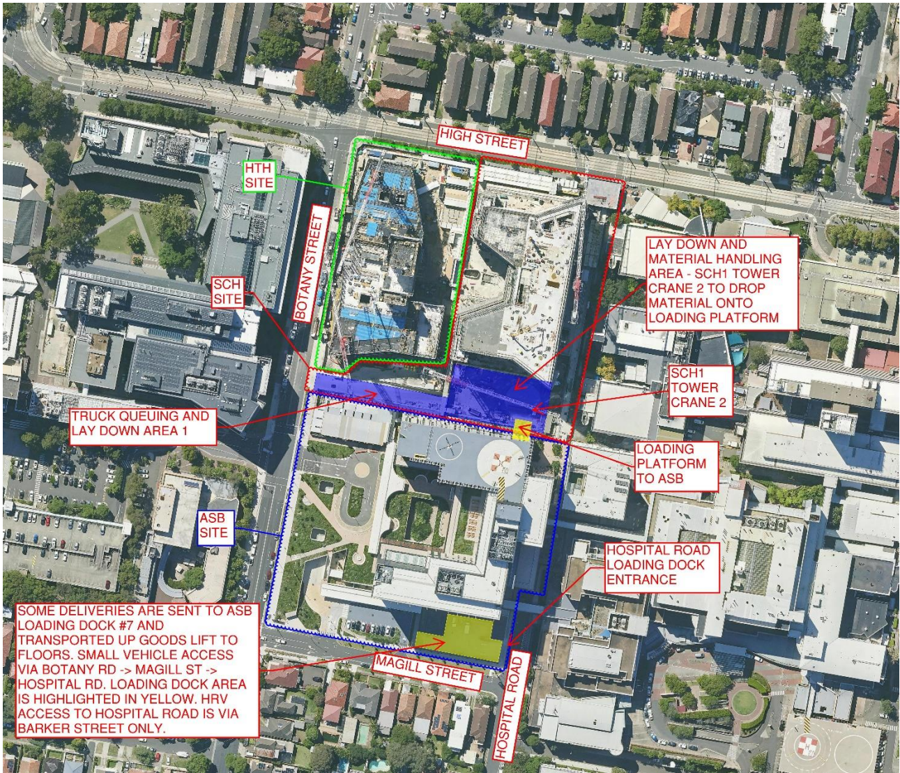
Figure 3 Site plan showing site access points for delivery and material handling area (John Holland)
